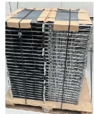
Products are secured to the pallet with tension straps. To protect the corners, they are protected with cardboard profiles.
